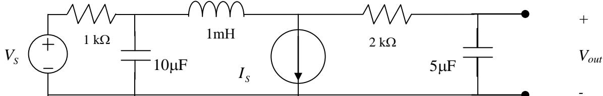
$$I_s = 0.001\angle 0, V_s = 2\angle 0^\circ, Z_L = j(10)(0.001) = j0.01, Z_{C1} = -j10k, Z_{C2} = -j20k$$
