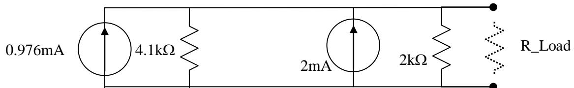
It now follows easily that  $I_{sc} = 2.98mA$ ,  $R_{TH} = 4.1k||2k = 1.344k\Omega$ ,  $V_{oc} = R_{TH}I_{sc} = 4V$
