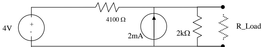
Apply a second source transformation to obtain a single node pair circuit
