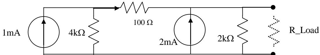
Simplify with a source transformation:  $I_s = 1mA$ ,  $R = 4k \Rightarrow V_s = 4V$
