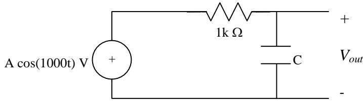
$$1. V_{out} = \frac{\frac{1}{jwC}}{R + \frac{1}{jwC}} V_{in} = \frac{1}{RCjw + 1} A\angle 0 = \frac{A}{\sqrt{R^2 C^2 w^2 + 1}} \angle -\tan^{-1}\left(\frac{RCw}{1}\right)$$
