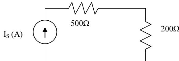
$$P_{200} = I_s V_{200} = I_s^2 200 = 1 \Rightarrow I_s^2 = \frac{1}{200} \Rightarrow I_s = \frac{1}{10\sqrt{2}} = \frac{1}{14.14} = 0.07(A)$$
