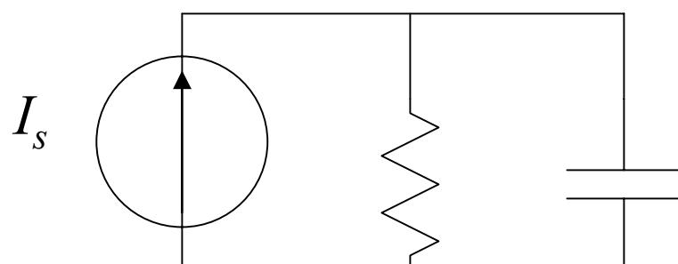
$$v_R = v_c \Rightarrow i_R = \frac{v_c}{R}; \quad i_R + i_c = I_s \Rightarrow RC \frac{dv_c}{dt} + v_c = RI_s$$
