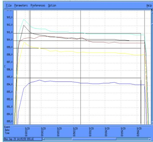
Figure 4. Detailed view of the top of the temperature ramp from figure 2, PID controller.
