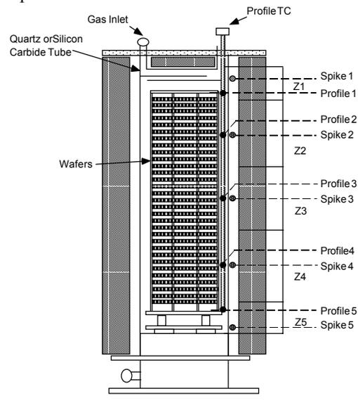
Figure 1. Schematic of a typical vertical furnace displaying the location of profile and spike thermocouples in relation to the heating element and wafers.
