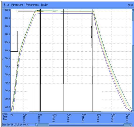
Figure 2. Oxidation process as controlled by the standard PID controller.
