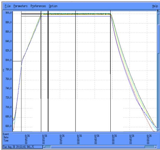
Figure 3. Oxidation process as controlled by the MBTC, displaying improved zone uniformity throughout the entire process.
