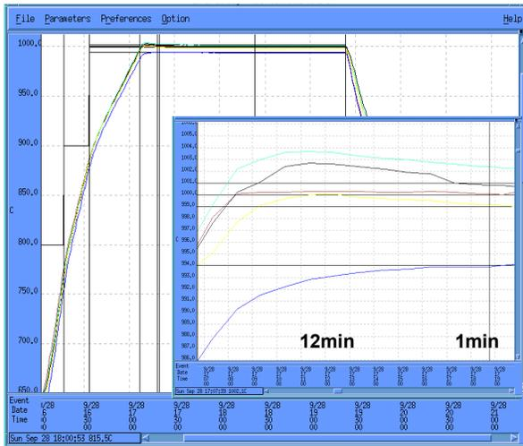
Figure 6. The maximized temperature ramp and stabilization time for the standard PID controller.
