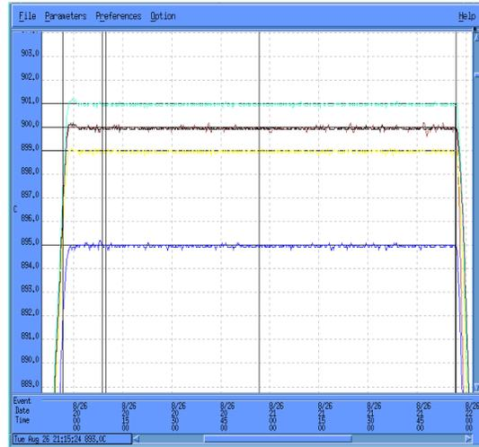
Figure 5. Detailed view of the top of the temperature ramp from figure 3, MBTC controller. The overshoot is virtually eliminated and the steady state control remains within  $\pm 0.1^\circ\text{C}$  during the entire process.
