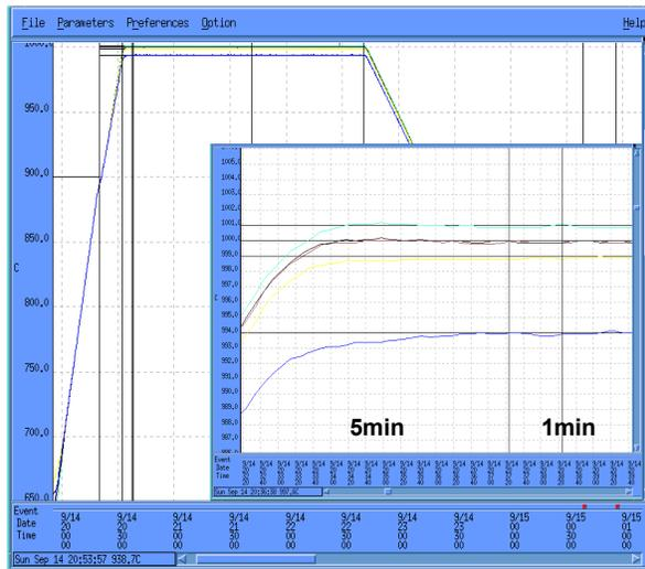
Figure 7. The maximized temperature ramp and stabilization time for the MBTC controller. The superb control of the MBTC allows for a faster ramp with less stabilization time.
